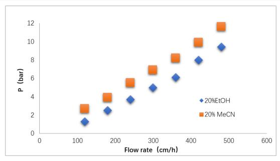
10\*600mm column Packing pressure: 5 bar
